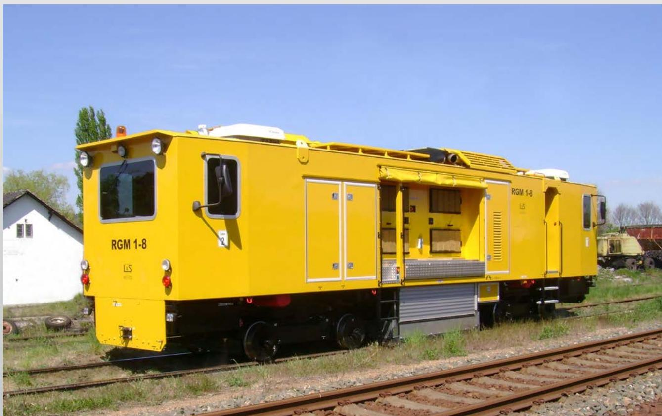
The rail grinder RGM 1-8 is a rail-borne machine which has 8 grinding spindles with independent angular adjustment. Each of the spindles is driven by a frequency-controlled electrical motor. The computer monitored grinding process is controlled with touch pad by the operator inside of the cabin.
