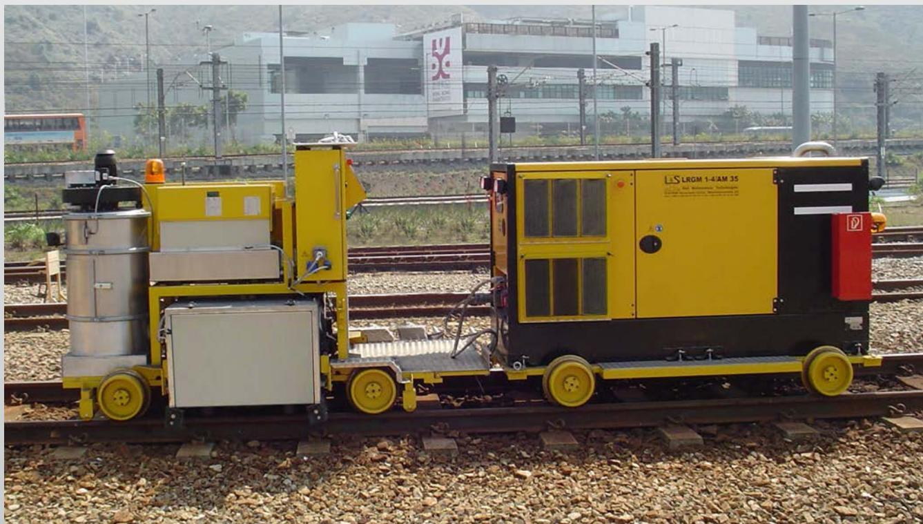
The LRGM 1-4/ AM35 is a turnout grinding machine for the machining of the rail head which composes except the grinding unit also a generator so that no power cables has to be installed along the working site. The grinder can be easily railed in and out with a ramp of a rail vehicle or by crane.
